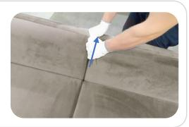
6. Spread the excess material over the edges of the backrest.
