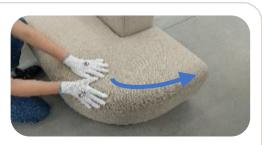
4. Move the creases formed at the curve of the seat backwards with your hands. If necessary slide the excess down the seat (towards the back).
